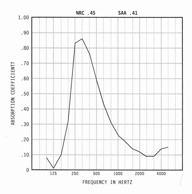
Specimen Area: 63.5 sq.ft. Temperature: 76.3 deg. F Relative Humidity: 42.0 % Atm. Pressure: 28.52 in. of Hg
